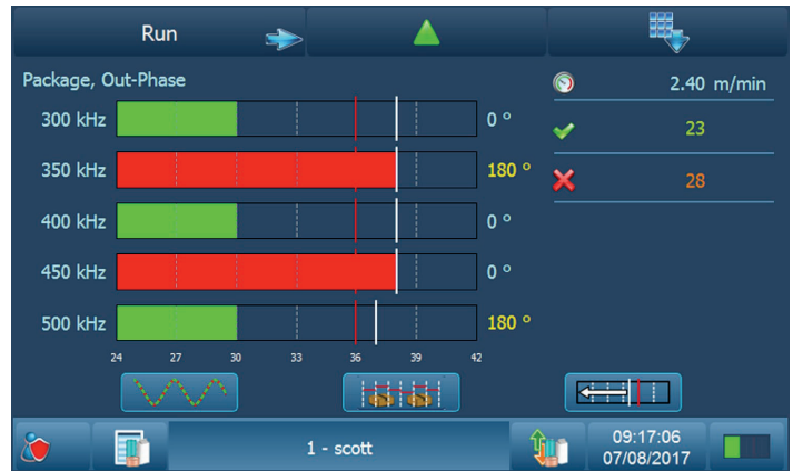
Results of each package at each Multiscan frequency are shown clearly on the Run screen
