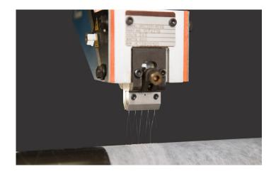
Rhythm construction nozzles deliver superior control of hot melt adhesive fiber size, density, and pattern width for numerous disposable hygiene and product assembly laminating applications.
