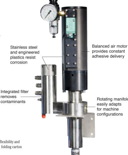
Nordson LA 300 dual-acting piston pumps offer flexibility and consistent high-flow rates of liquid adhesives in folding carton and bag and sack manufacturing.
