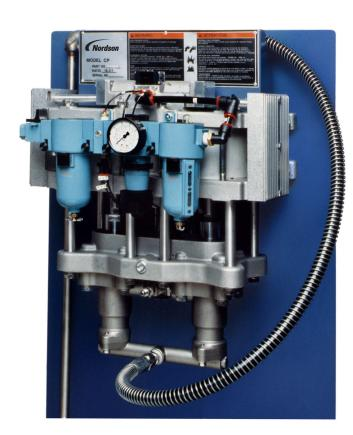
The Nordson Model CP (Constant Pressure) Pump is an air-driven pump for the application of container coating materials in both heated and unheated delivery systems. Developed specifically for the container industry, the demand-type, dual=piston CP Pump maintains constant fluid pressure throughout the pumping operation for superior overall performance necessary in high-speed can coating applications.
