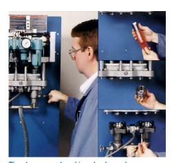
The plungers and packing glands can be easily replaced on-line in 20 minutes.
