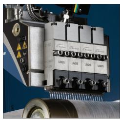
Mix and match bead inserts to meet required pattern compression and bond strength.
