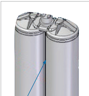
Separate bores, CL 0.7mm wider
