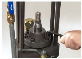
Packing gland is easily removed without special tools
